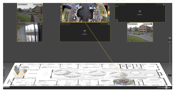
The map can contain icons for cameras, relays, and sensors. The area in which live video is displayed and field of view are indicated for each camera.
