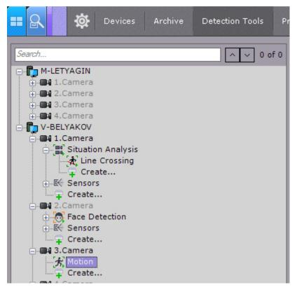
To create a detection tool, click Create in the camera's object tree and choose a required tool.
