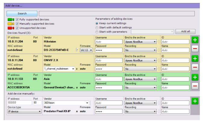
The IP devices are color-coded based on the status of the device.
