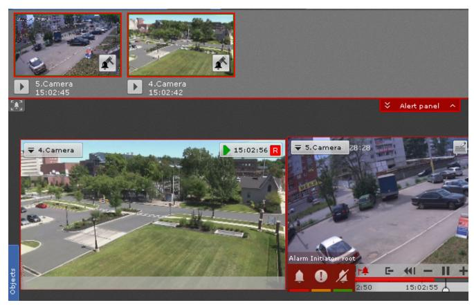
When you classify an alarm (critical, non-critical, false, or missed), a flag is added to the alarm recoding on the timeline. A flag is added to the point on the timeline when the alarm began.
